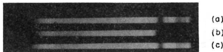
Fig. 4.—Typical spectra on hypersensitized Kodak IIL emulsion through glass optical system: (a) flash before irradiation through 0.5 M \text{Na}_2\text{CO}_3 solution; (b) flash simultaneous with electron pulse; (c) flash 30 sec. after electron pulse.
